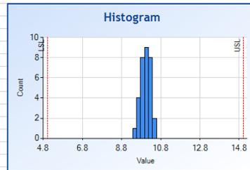
GageStudy performs a Type 1 Gage Study on a single sample of gage data to check its suitability to make capable measurements considering the gage spec limits and a reference standard. The above two charts show the variability of the gage being studied as a RunPlot and as a Histogram. The GageStudy report among other items, the Gage capabilities Cg (variability only) and Cgk (variability considering the mean relative to the standard reference).
