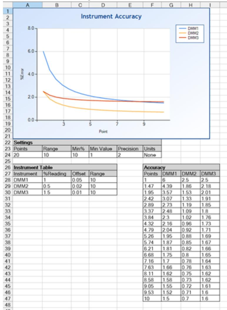
The InstrumentsAccuracy chart type is a tool to characterize the accuracy of measuring instruments over a specified range based on %Reading Error, Offset Error and Range. The tool can be used to characterize a single instrument, or multiple instruments performing the same task to compare capabilities. The latter is useful if multiple manufacturers/models are being considered, and it is desired to select the best one for the task and cost.
